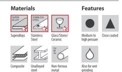
Universally usable silicon carbide abrasive belt with high cutting capacity and wide range of grit sizes. Achieves a fine scratch pattern and ensures particularly brilliant gloss levels (high gloss unit). Since CK721X is oil- and water-resistant, the gloss level can be further increased by using grinding oils.
