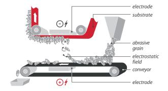
The principle of electro static coating
